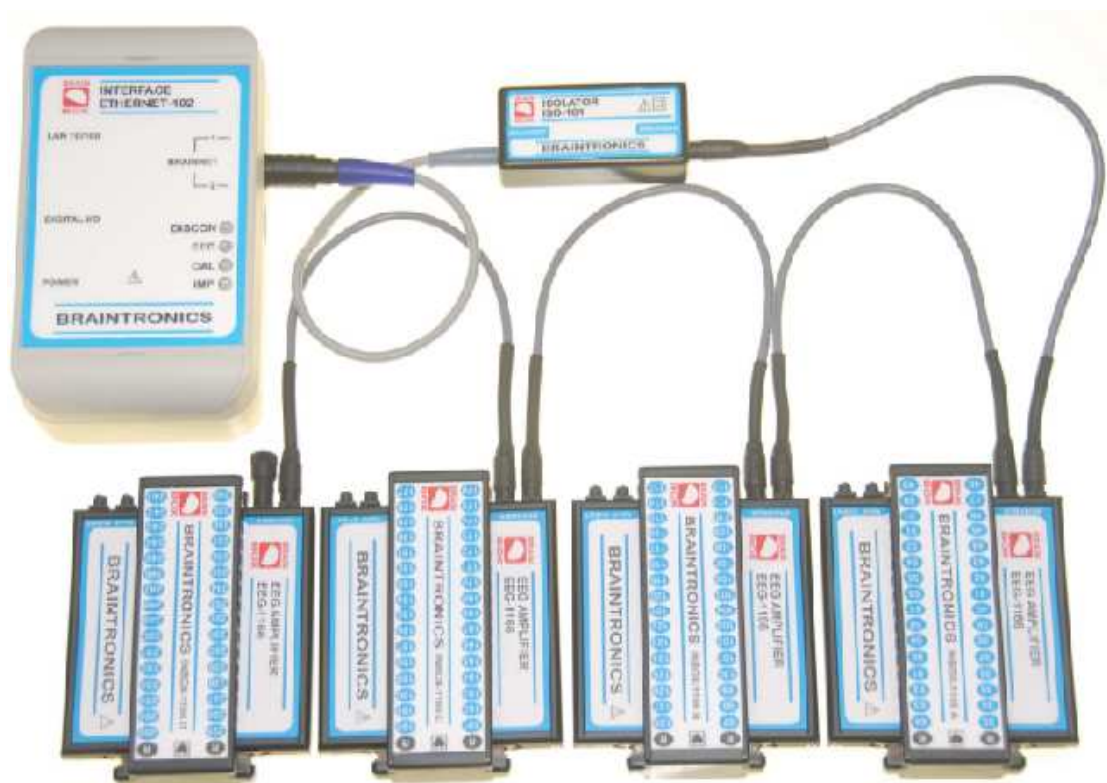
Photo of maximum 256 Ch. system using 4 BRAINBOX® EEG-1166 amplifiers.
